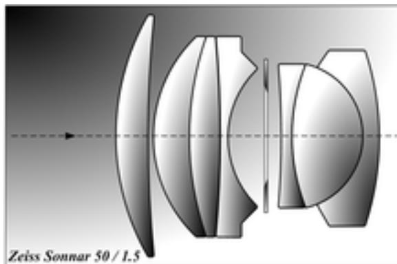
This diagram of the Zeiss Sonnar 50mm f1.5 has 7 optical elements in 3 groups. The Sonnar was first introduced in the 1930s and was known for its sharpness and light weight. Some variable focal length lenses have as many as 20 elements!
